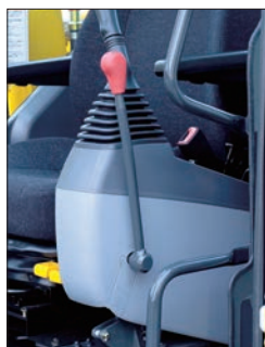
Lever shown in lock position
